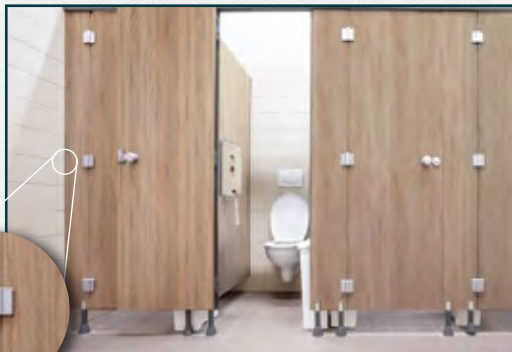
TRADITIONAL CONSTRUCTION (Exposed hinges for outward opening ambulatory cubicles)
