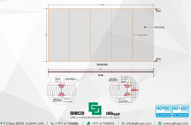
Correction of uneven floor and ceiling levels up to ±10mm.
